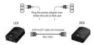
Note: Flexible power is different from Power over Ethernet (PoE). Ensure the CAT 5e/6/7 cable is only connected between the LEX and REX units.
